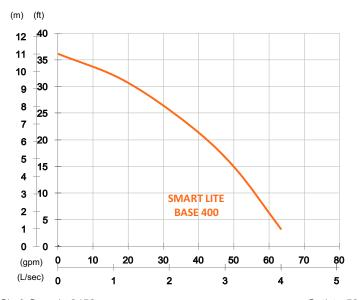
Shaft Speed: 3450 rpm Outlet: 50mm, 2in
